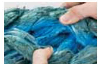
Inspect for internal abrasion.
