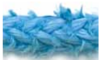
Severely abraded rope.
