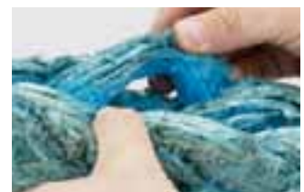
Inspect for pulled strands.
