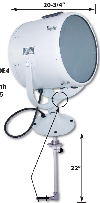
Fig. 1902 Light Shown With Fig. 1921 Lever/Gear Control
