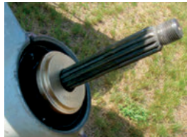
Fig. 7 The forward thrust washer is tapered and will nest with the taper on the propeller shaft. When properly installed, the part number will be visible.
