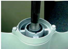
Fig. 5 Propeller shaft taper is visible, indicating OEM forward thrust washer has been removed. XHS Hub Kit forward thrust washer ready to be installed.
